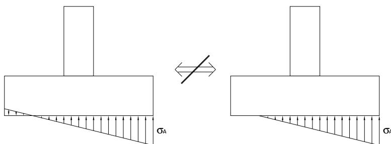
There are two correct solutions in the design of a foundation. The classical approach is to increase the size of the footing until the uplift is 0, but this may lead to overdimensioning. The most economical way to calculate a foundation, is to consider the uplift.
